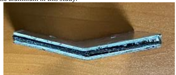
Figure 9. Al+C+Al (t=4.5 mm) for 20 mm mold width at 150° bending angle
