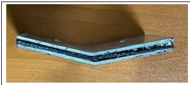
Figure 9. Al+C+Al ( t=4.5 mm) for 20 mm mold width at 150^\circ bending angle.
