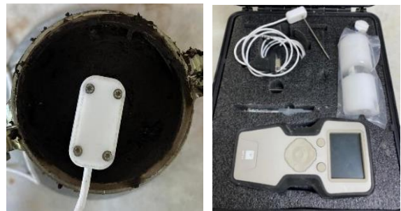
Figure 7. TEMPOS thermal properties analyzer.
