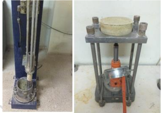
Figure 6. Standard Proctor test equipment.
