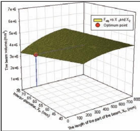
Figure 4. The objective function versus design variables with the optimum point.
