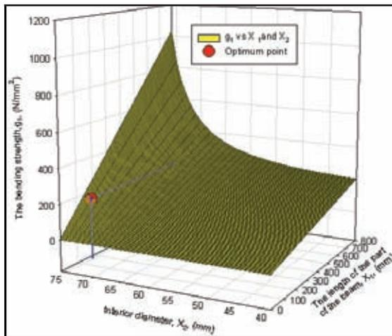
Figure 5. The design variables versus inequality constraint, with the optimum point.
