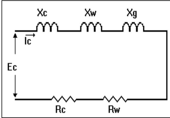
Figure 5. Electrical equivalent circuit of an induction heater coil
