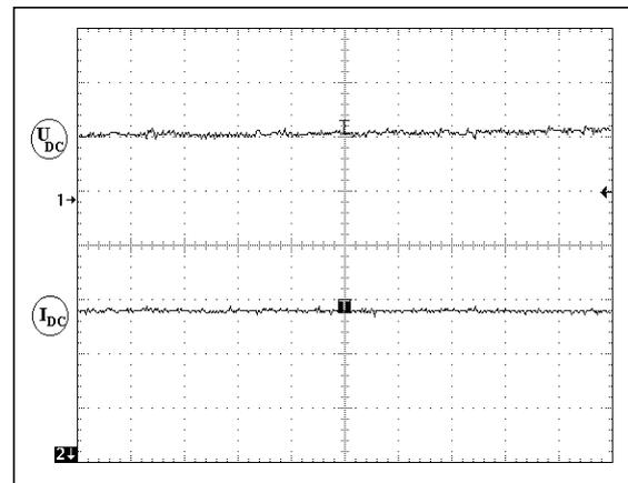
Figure 6 Measured input DC line voltage [CH1:100V, CH2:1A, T:20μS].
