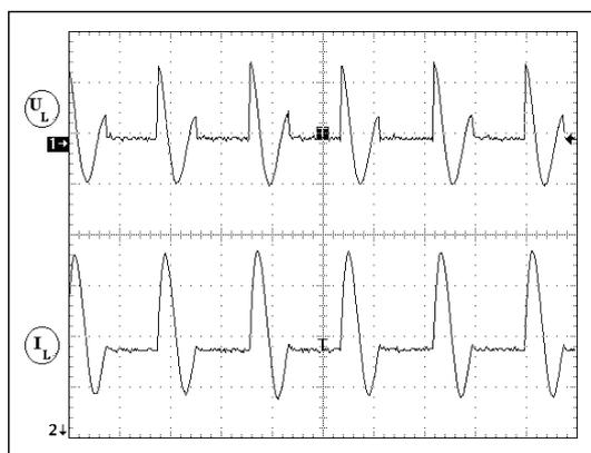
Figure 8. Measured load voltage  $v_L$  and load current  $i_L$  [CH1:50V, CH2: 5A, T: 0.5mS]
