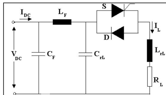
Figure 1. Circuit diagram of the proposed induction heating system
