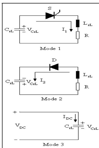
Figure 3. Equivalent modes of operation
