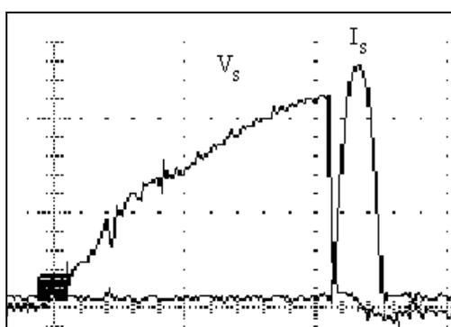
Figure 4. Switch voltage  $V_S$  and current  $I_S$  waveforms during turn-off
