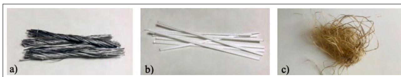
Figure 1. Fibres types. a) Copolymer fibre, b) Polypropylene fibre, c) Hemp fibre.
