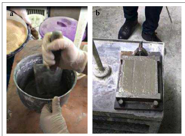
Figure 2. (a) Mixing with a trowel (b) Compacting mortar B.
