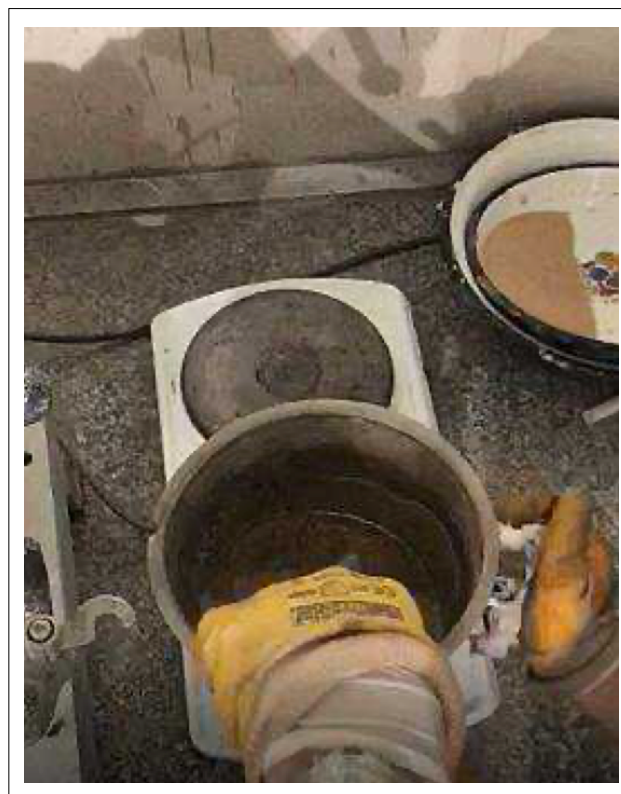
Figure 3. Electric stove used during the production of sulfur mortar.
