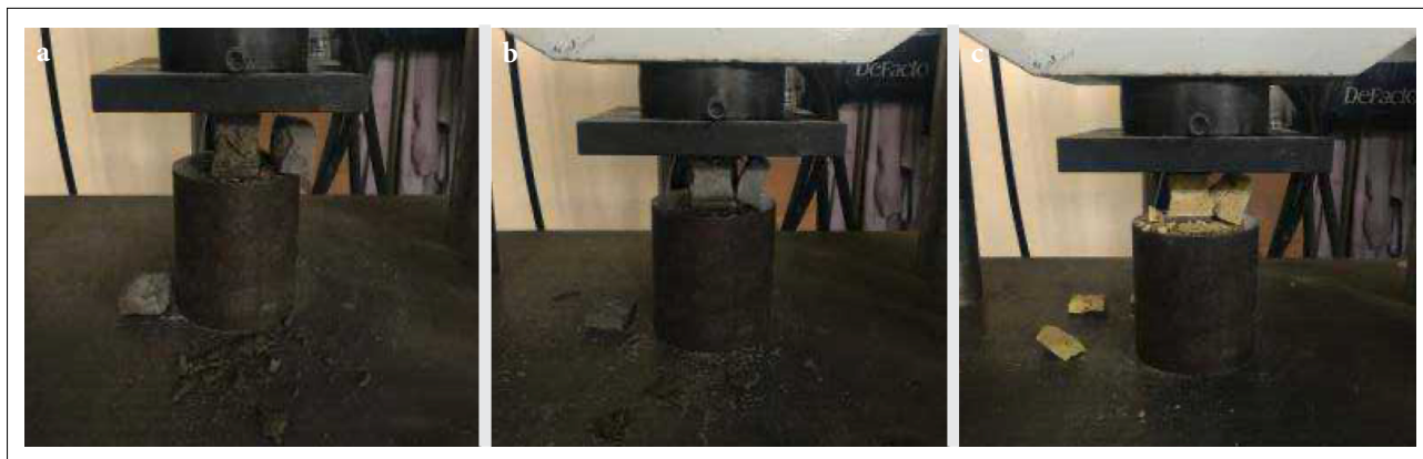
Figure 8. Compressive test of three different mortar samples (a) A mortar (b) B mortar (c) C mortar.
