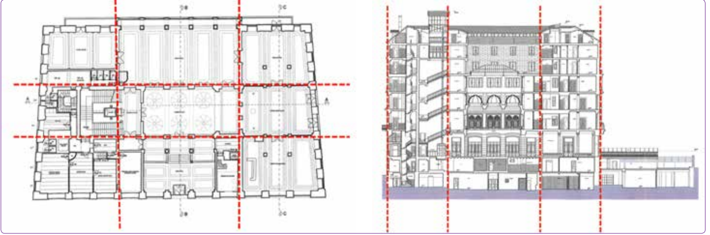
Figure 5. Structural axes on ground floor and longitudinal section.
