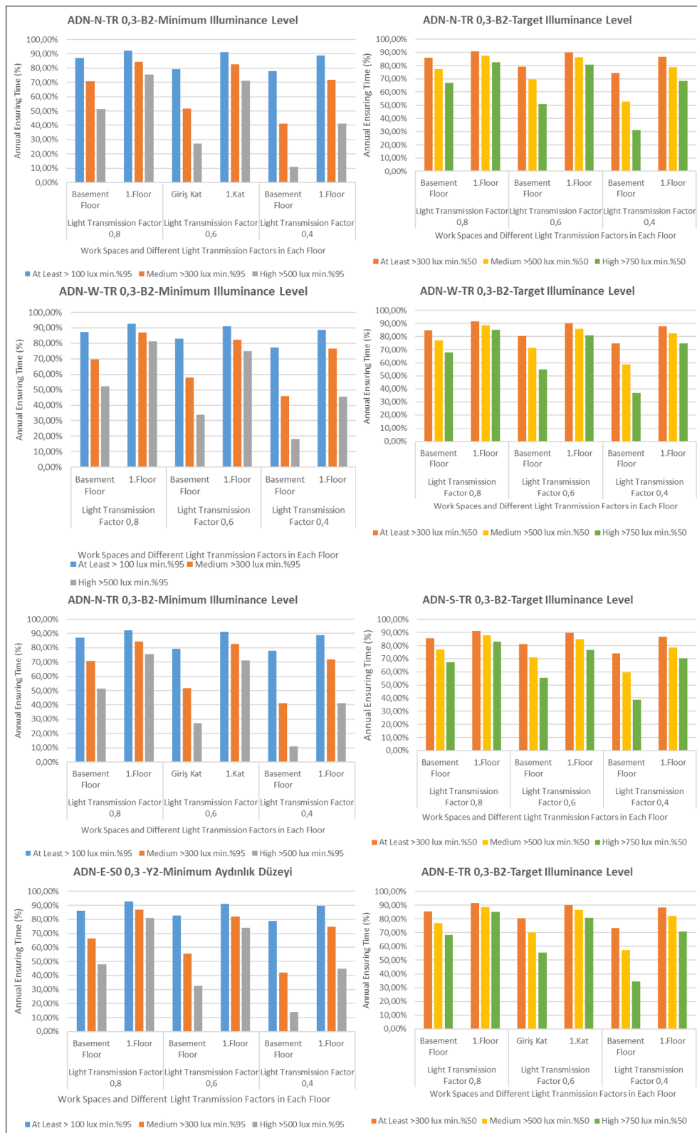
Figure 3. Annual ensuring time of minimum and desired illuminance levels for ADN-B2 N,E,S,W-LTF 0.8,0.6,0.4 and TR 0.3 in workspaces on each floor (%).
