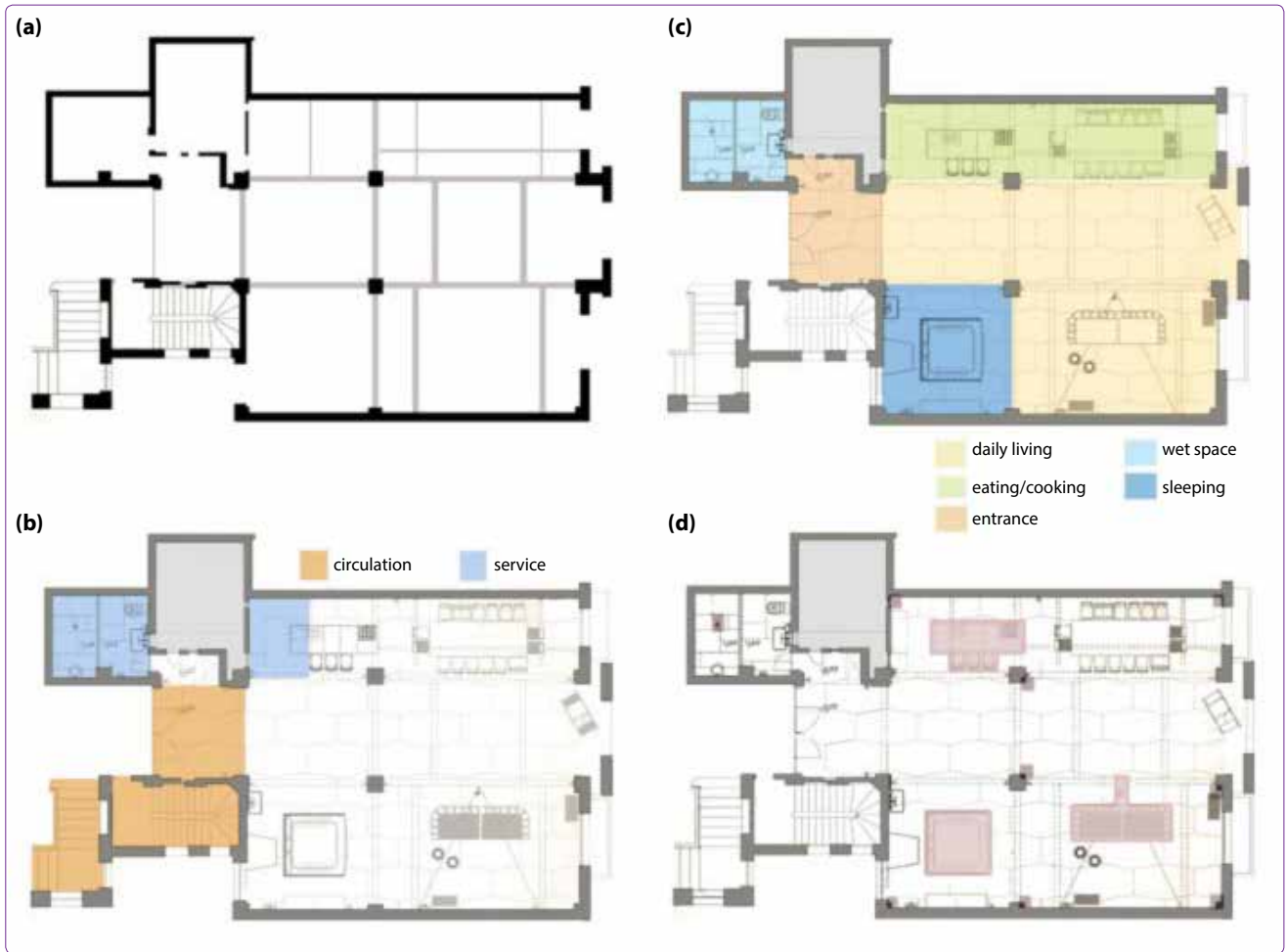
Figure 7. (a) Structure; (b) Service; (c) Spatial Organization; (d) Furnishing. ( Misir Loft , 2004. Tasarım Dergisi , vol.147, pp.132-139. Figures of case studies' analyses (Fig. 3-8) are edited by the authors. Last accessed date is 15.08.15 for all web sources.)
