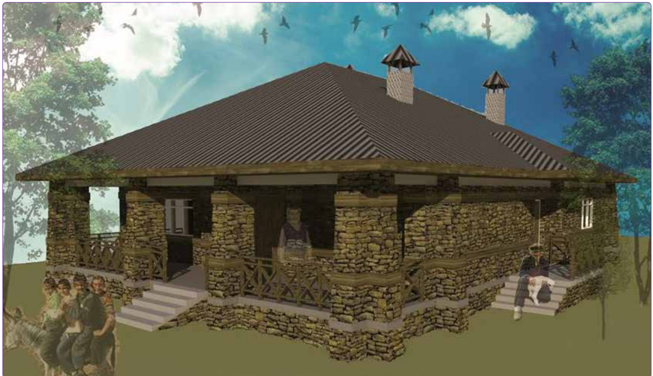
Figure 17. Suggested masonry house of pilot region with props and reinforced-concrete beams (Prepared by Author and members of Workshop, 2012).
