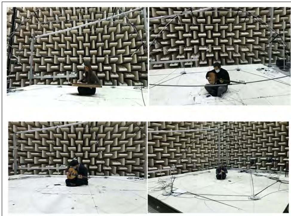
Figure 4. Directivity measurements of instruments.
