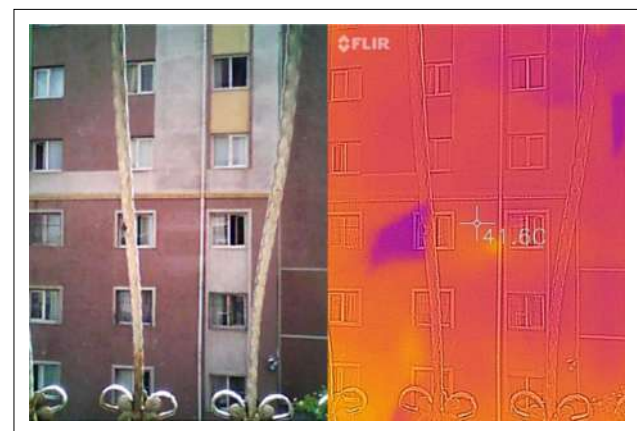
Figure 10. Exterior wall temperature on the southeast façade of Block 3 in TOKI Etiler in July (Photo by Bay-Şahin, 2019).
