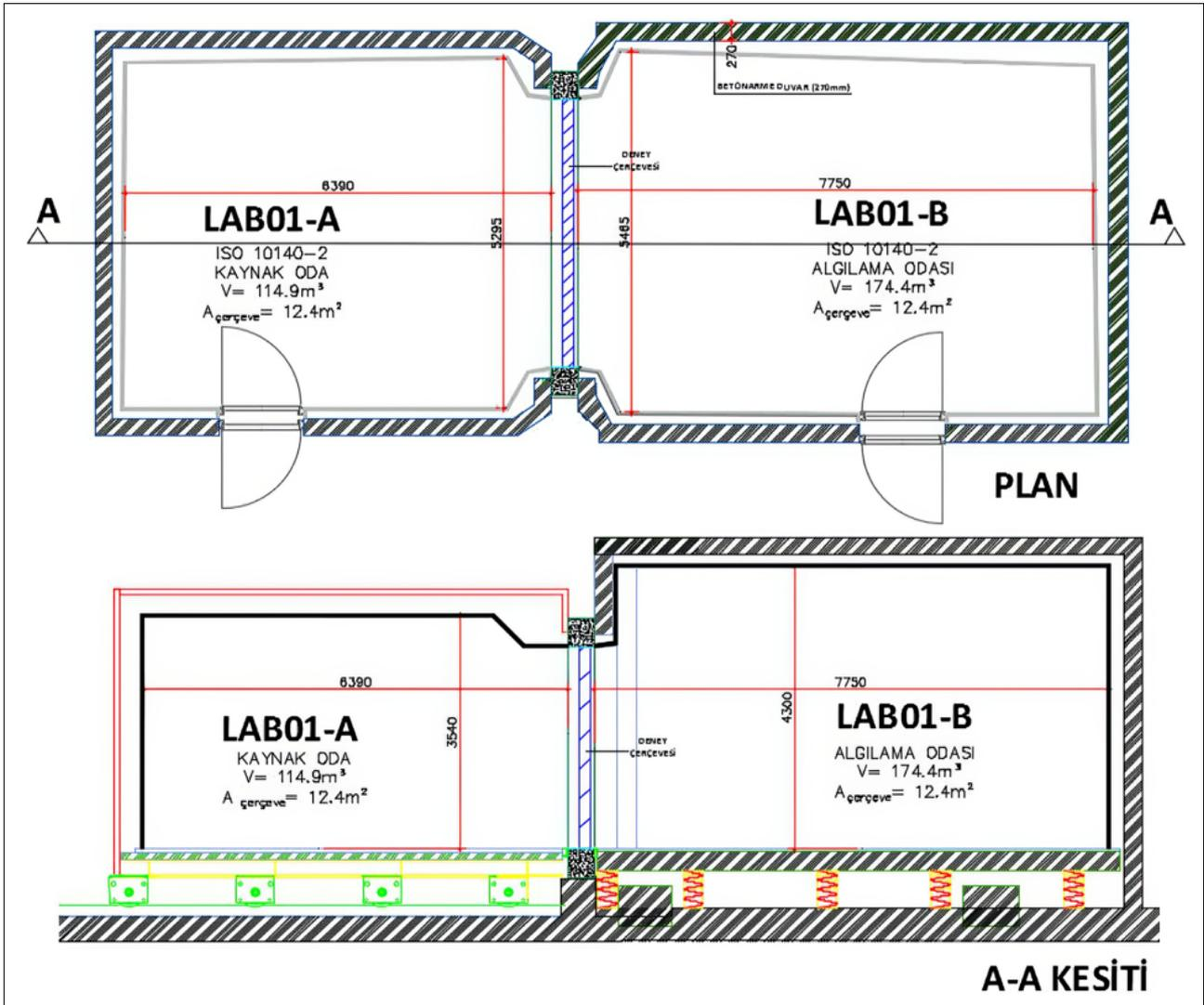
Figure 4. Section and Plan Views of the Test Room.
