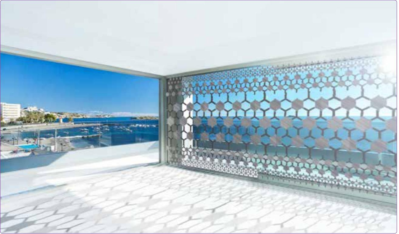
**Figure 34.** RRPS application as an exterior sun shade for a building facade.
