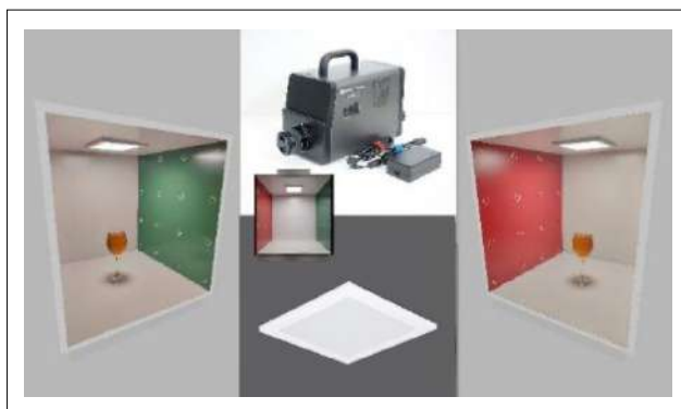
Figure 2. Experiment box, luminaire, spectroradiometer, and liquids.
