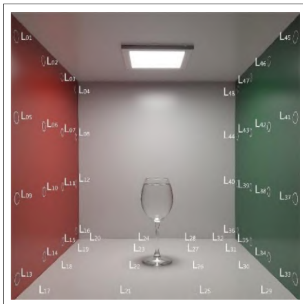
Figure 6. Experiment box and measuring points.
