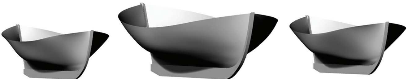
Figure 6. The hull models of the Tirhandils, numbered T-1, T-2, T-3 (from left to right)
