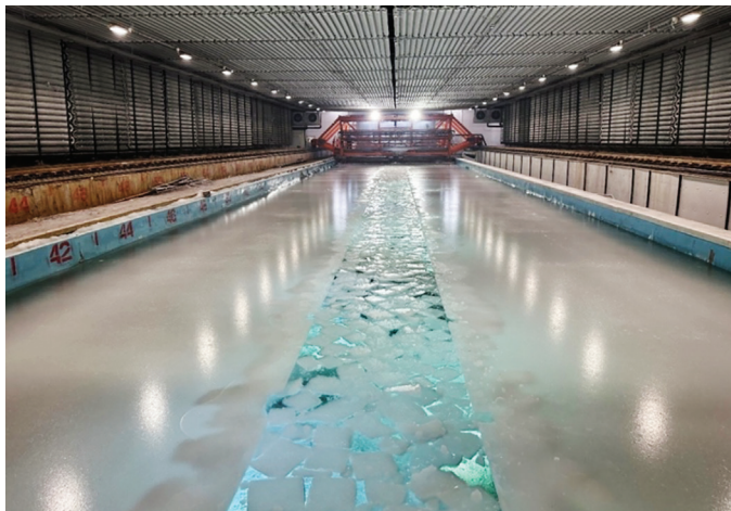
Figure 1. Model ice channel filled with broken ice (concentration 9/10)
