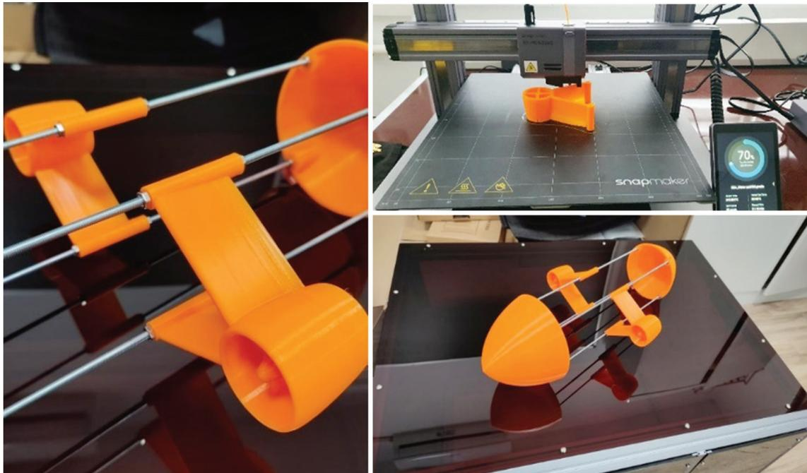
**Figure 12.** Stages of printing and installation of AUV propulsion engines
