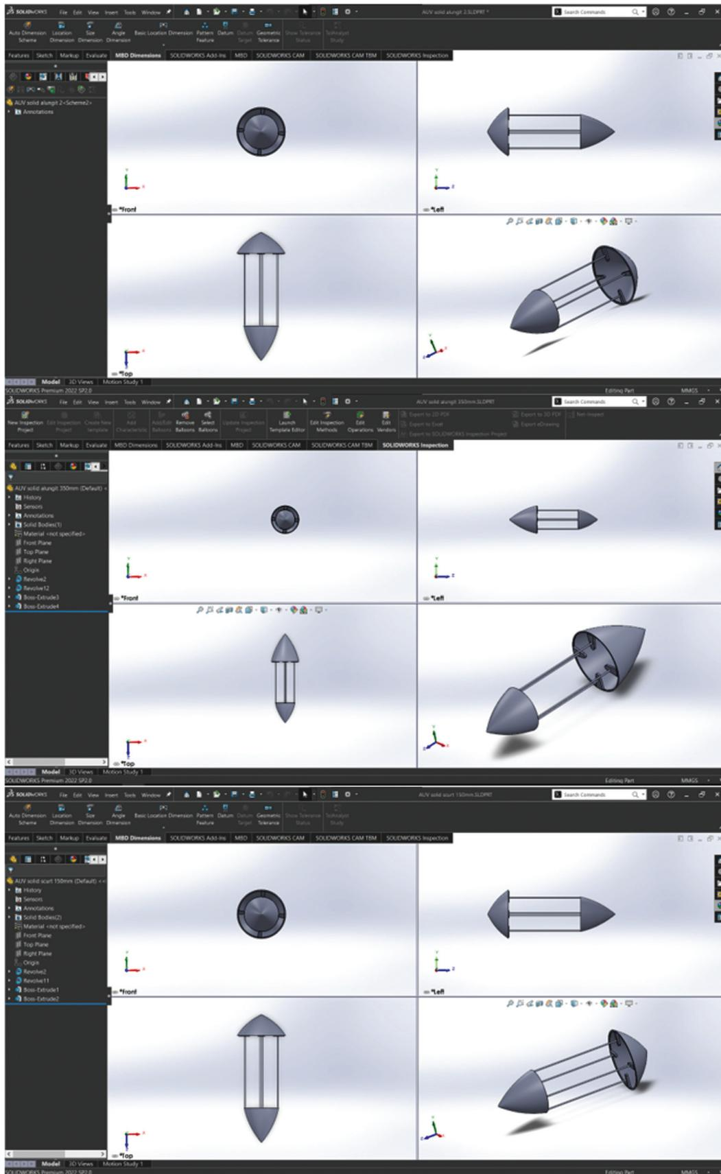
**Figure 3.** Shape variants for AUV
