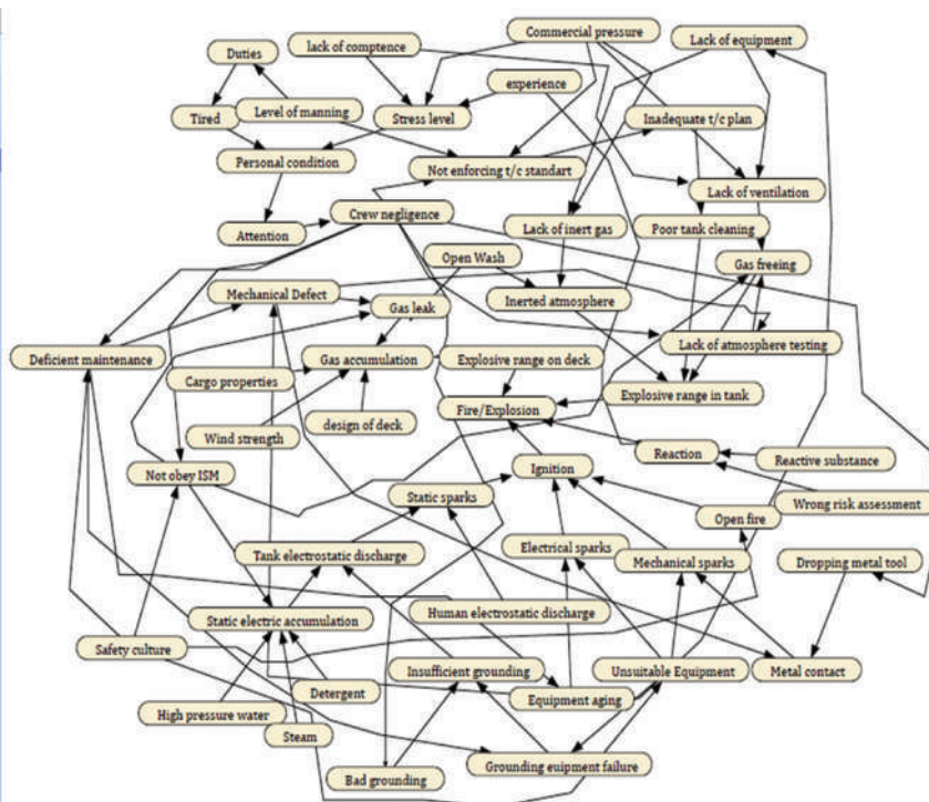
Figure 3. Fuzzy Bayesian Based Safety Assessment Model for Tank Cleaning Operation on Oil/Chemical Tanker
