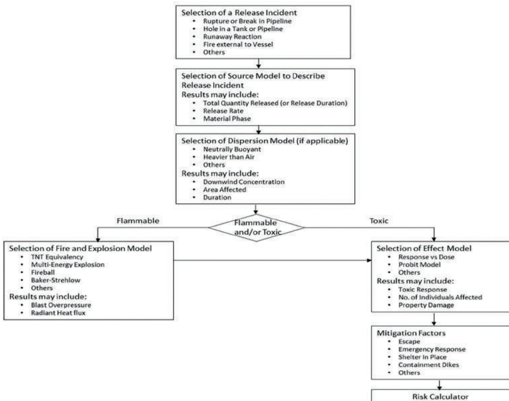
Figure 1. Logic Diagram for Consequence Models due to Releases of Volatile Hazardous Substances [12]
