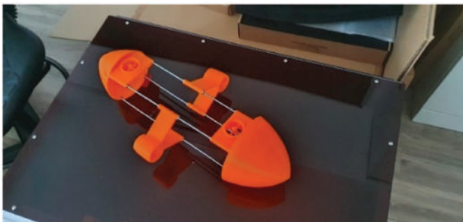
Figure 13. Autonomous underwater vehicle-3D printed prototype produced quickly and with free market equipment resulted in the context of the presence of sea mines in areas of national responsibility in the Black Sea (in the context of the armed conflict between Russia and Ukraine) and the lack of the expected final result from the MAS-MCM project. Under these conditions, the Romanian National Naval Forces were forced to intervene in the discovery and destruction of sea mines using non-compliant resources (ships from the military fleet), thus exposing both ships and personnel to very high risks.
