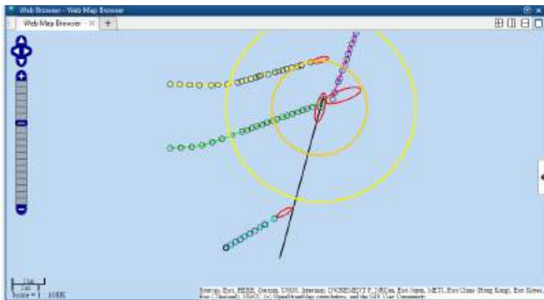
Figure 12. The path followed by own ship for the vessel crossing Stand-On (Rule 15)
