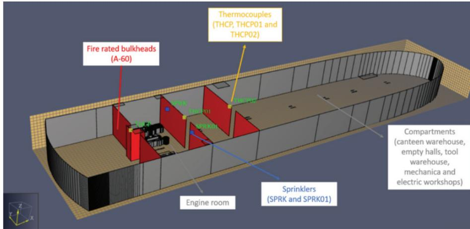
**Figure 4.** Geometric model structure of the lower deck of SH SUTLUCE
