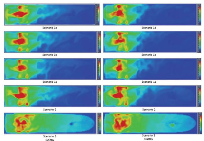
**Figure 19.** Temperature distribution on  $z=2.8$  m at  $t=100$  s and  $t=200$  s for all scenarios
