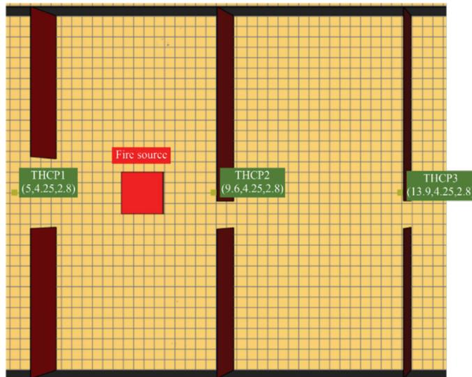
Figure 11. Arrangement of thermocouples in the lower deck
