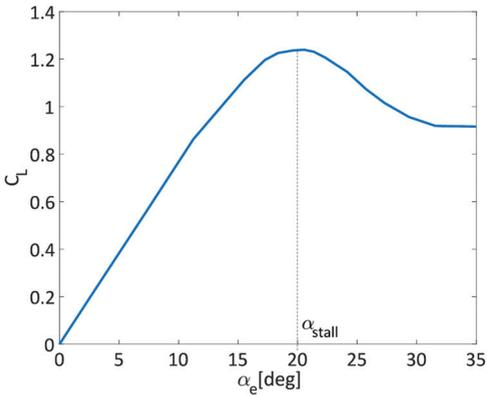
Figure 1. Steady Free-stream Lift Characteristic of the Fin
