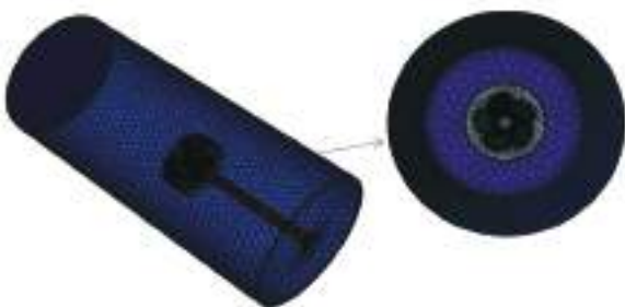
Figure 4. Meshing configuration of the B-5 propeller
