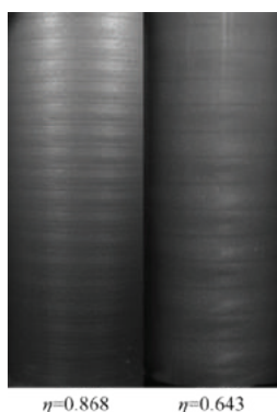
Figure 3. Formation of Taylor Vortices in TVF in Narrow and Wide Gaps
