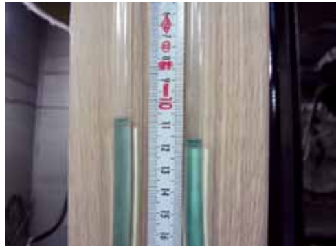
Figure.11 Visual pressure drop measurement, U-manometer.
