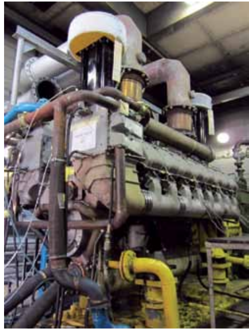
Figure.10 Shop trial tests at TULOMSAŞ factory.
