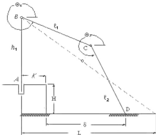
One major design objective for the arm is to be able to reach, via an unshown gripper located at the end D, an object located at ground level and within a working radius L (Figure 2). Hence, lengths of the links need to be selected so that the entire working length L-K is accessible to the arm at ground level.
