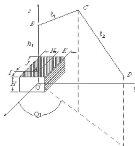
In what follows, a three-link arm is considered, as shown in Figure 1, with three revolute joints. Work space constraints are set and relationships are formulated that enable the determination of link dimensions to meet the constraints. Likewise, relationships are set up between locations of the work piece and displacement variables.
