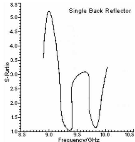
Table 4 shows the variation of main to side-lobe level ratio and half power beam width with frequency for the double back reflector backfire antenna in the E-Plane. Table 5 gives a comparison summary for the performance of the double back reflector backfire antenna, the single back reflector backfire antenna and the aperture. Figures 4 and 5 show the variation of S-ratio with frequency for the two antenna types.
