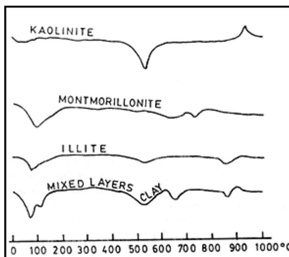
Figure 2: Thermograms of Typical Clays.
