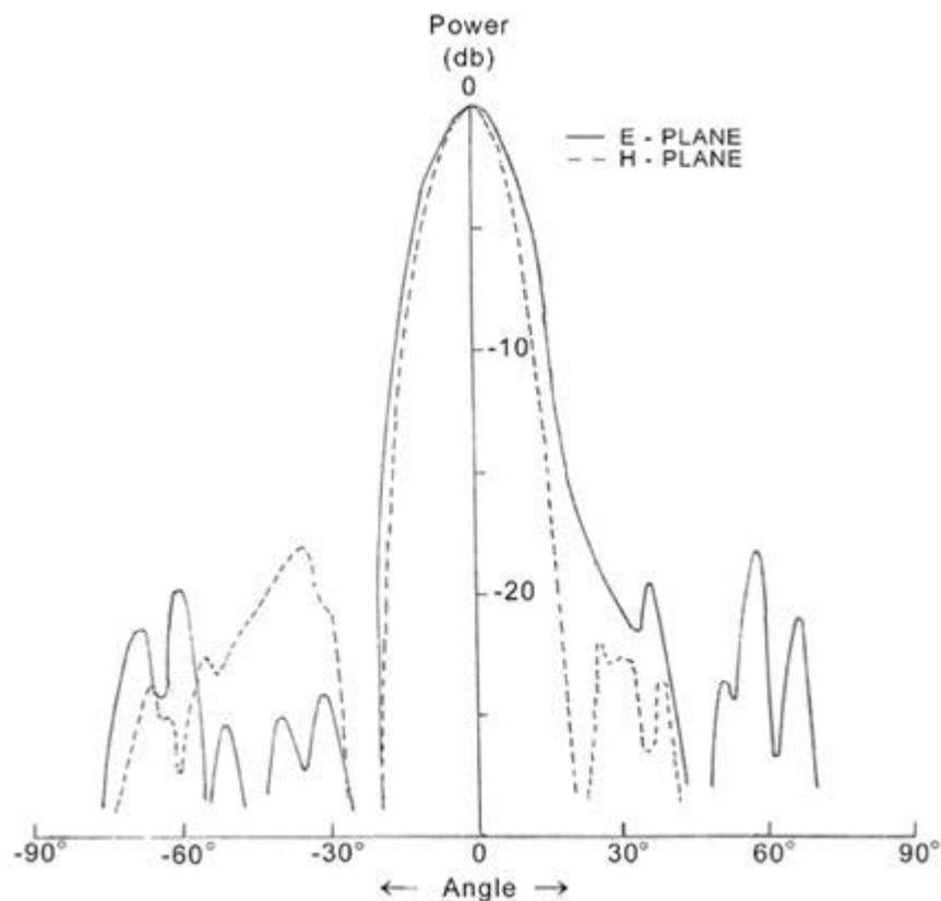
planes and that the highest values of the antenna under test gain is 17.2 db which is generally higher by 1.0 db where compared with the antenna of one small front circular disk, and about 6 db over the cup antenna (10), where the other parameters were shown in Table 2.
