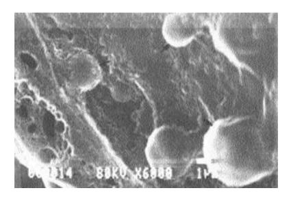
size of CaF<sub>2</sub> deposits in the surface coating produced by topical fluoride agent may be an important factor in determining the effectiveness of a topical fluoride agents. As the solubility of crystals decrease with their increasing sizes, CaF<sub>2</sub> particles occurring as a result of APF application will dissolve slower than those of NaF application.
