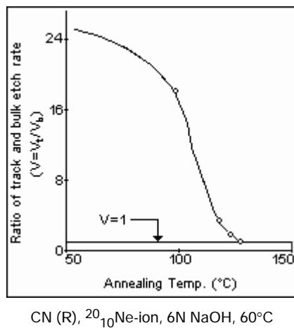
perature as shown in Figure 8. It is observed that  $V_t$  decrease with annealing temperature.
