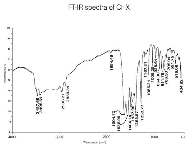
**Figure 2.** FT-IR spectrum of CHX molecule was obtained by FT-IR databases.<sup>24</sup>
