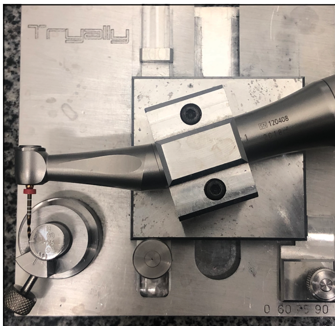
Figure 1. The instrument positioned in the cyclic fatigue test device showing the artificial canal with an angle of curvature of 60° and a radius of 5 mm
