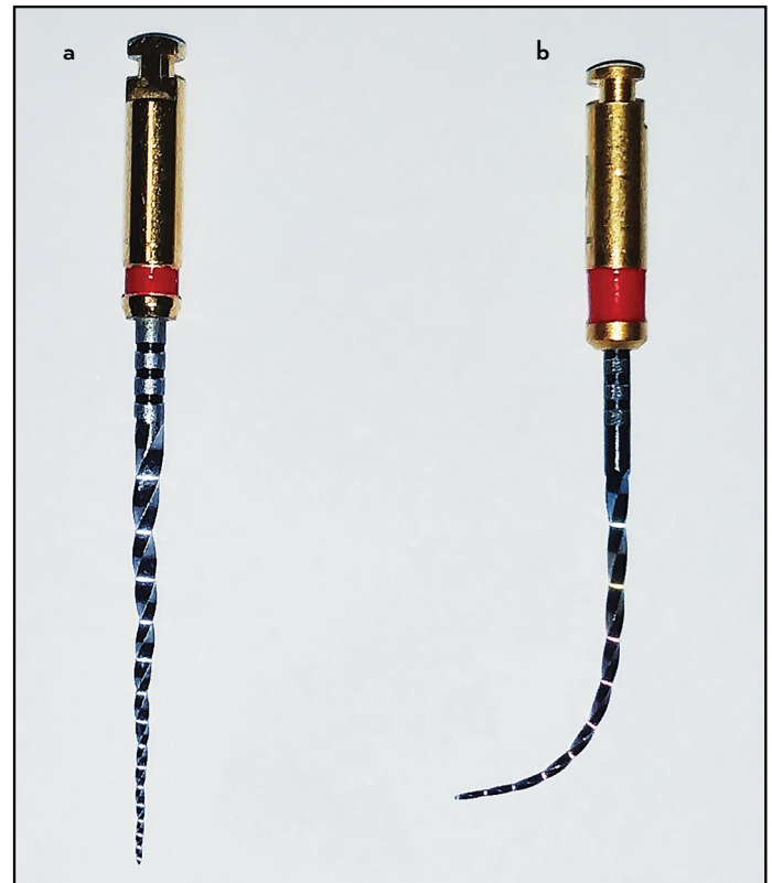
Figure 3. Comparison of austenitic (ProTaper Next) and martensitic NiTi files (CM wire). (a) The austenitic NiTi file cannot be bent at room temperature; (b) The martensitic file can be bent at room temperature
