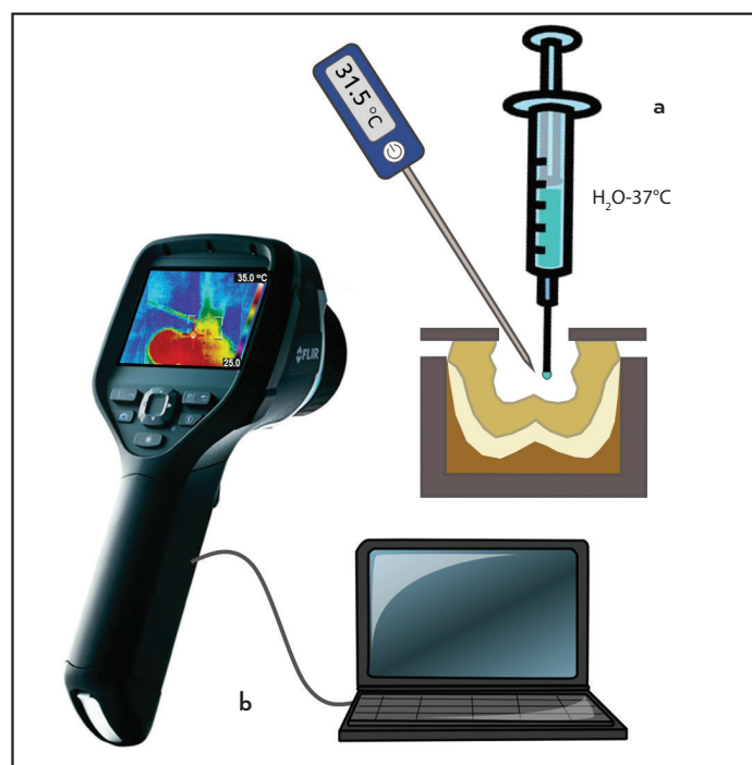
Figure 1. Experimental preparation for thermographic video recording in the simulation of a tooth with vital pulp tissue (a) Perfusion system (syringe with warm water) and thermocouple inside the tooth (b) Thermographic camera (left) connected to a computer (right) for image recording
