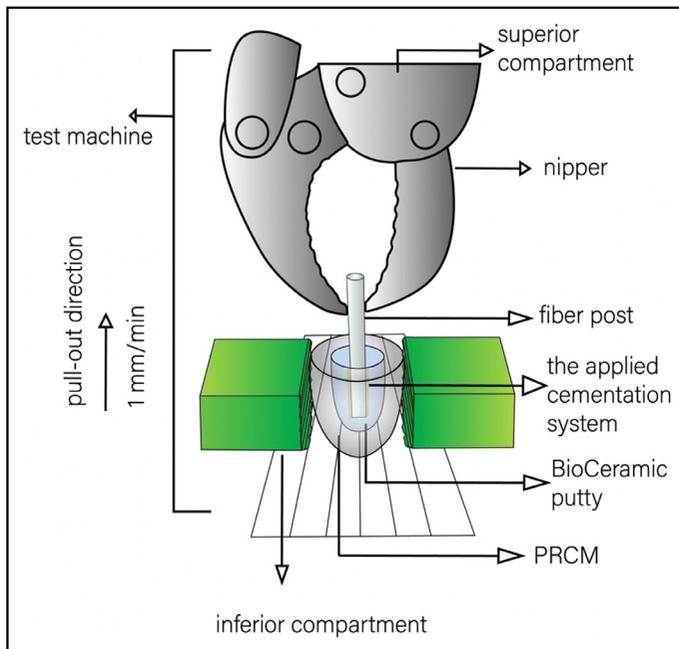
**Figure 5.** Schematic diagram of pull-out test set-up
