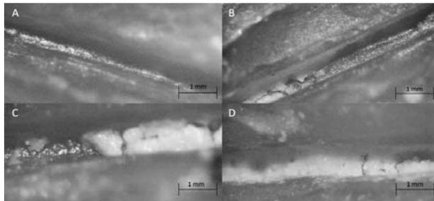
**Figure 1:** Groove scores (A) Score 0: the groove is empty; (B) Score 1: less than half of the groove is filled with debris; (C) Score 2: more than half of the groove is filled with debris; (D) Score 3: the complete groove is filled with debris. Original magnification, 40x.
