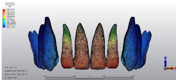
Figure 12. Frontal view of movements occurring in the “Y” axis
