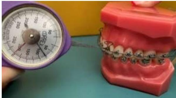
Figure 9. Application of the asymmetrical T-loop to the typodont model and measurement was done from the mesial of the lateral bracket with the help of a force gauge. The force gauge shows 75 grams of force.
