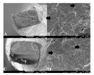
Fig. 2. Scanning electron microscopic images of fractured surfaces of WaveOne Gold Primary (A-B) and Hyflex EDM OneFile (C-D) instruments show typical features of cyclic
