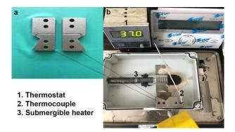
**Fig. 1.** Artificial canal block with abrupt apical curvature (a) Static cyclic fatigue test device simulating body temperature (b)
