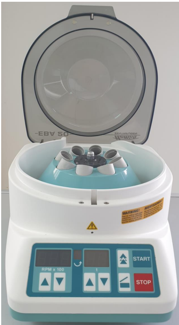
Fig. 2. Centrifugation machine used to centrifuge and produce any types of platelet concentrates
