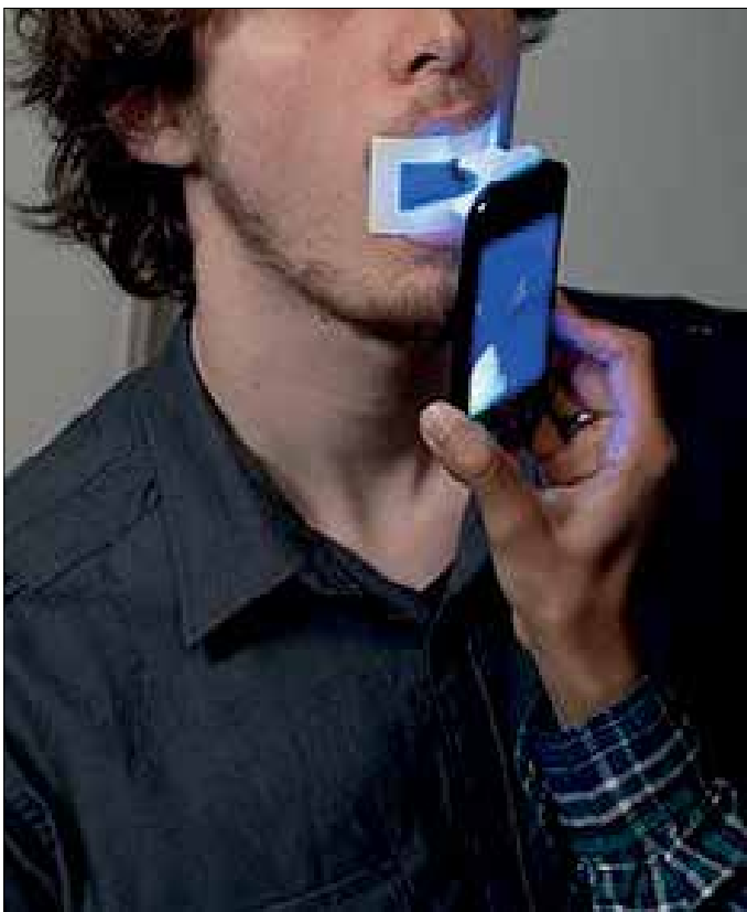
Figure 3. OScan® contains two rows of fluorescent light-emitting diodes that illuminate the mouth and highlight lesions and dark spots
