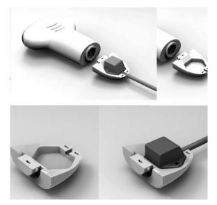
Figure 1. Tracking sensor embedded in the ultrasound probe mock-up.
