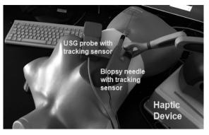
Figure 2. Ultrasound probe and biopsy needle with embedded trackers and the haptic device connected to the biopsy needle.
