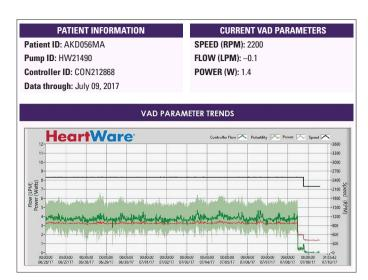
Figure 1. HVAD parameters and flow pulsatility over the last 14 days
