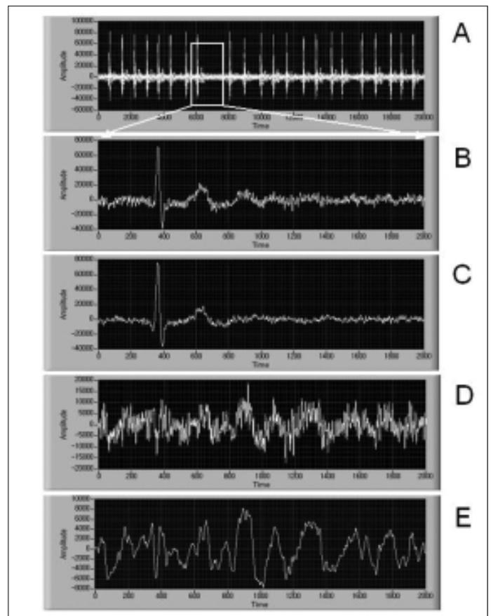
**Figure 3. Example of signal processing of AF activity recorded with unshielded MCG (courtesy of Dr. K. Kim; see ref 33, 34). A) Raw data (one MCG channel). B) Selection of a long cardiac cycle with minimal overlapping of QRS on AF waves. C) QRST separation with ICA. D) Amplification of AF waves after QRS subtraction. E) Low-pass filtering (20Hz). The signal-to-noise ratio achieved is more than adequate for the beat-to-beat study of AF activity.**
