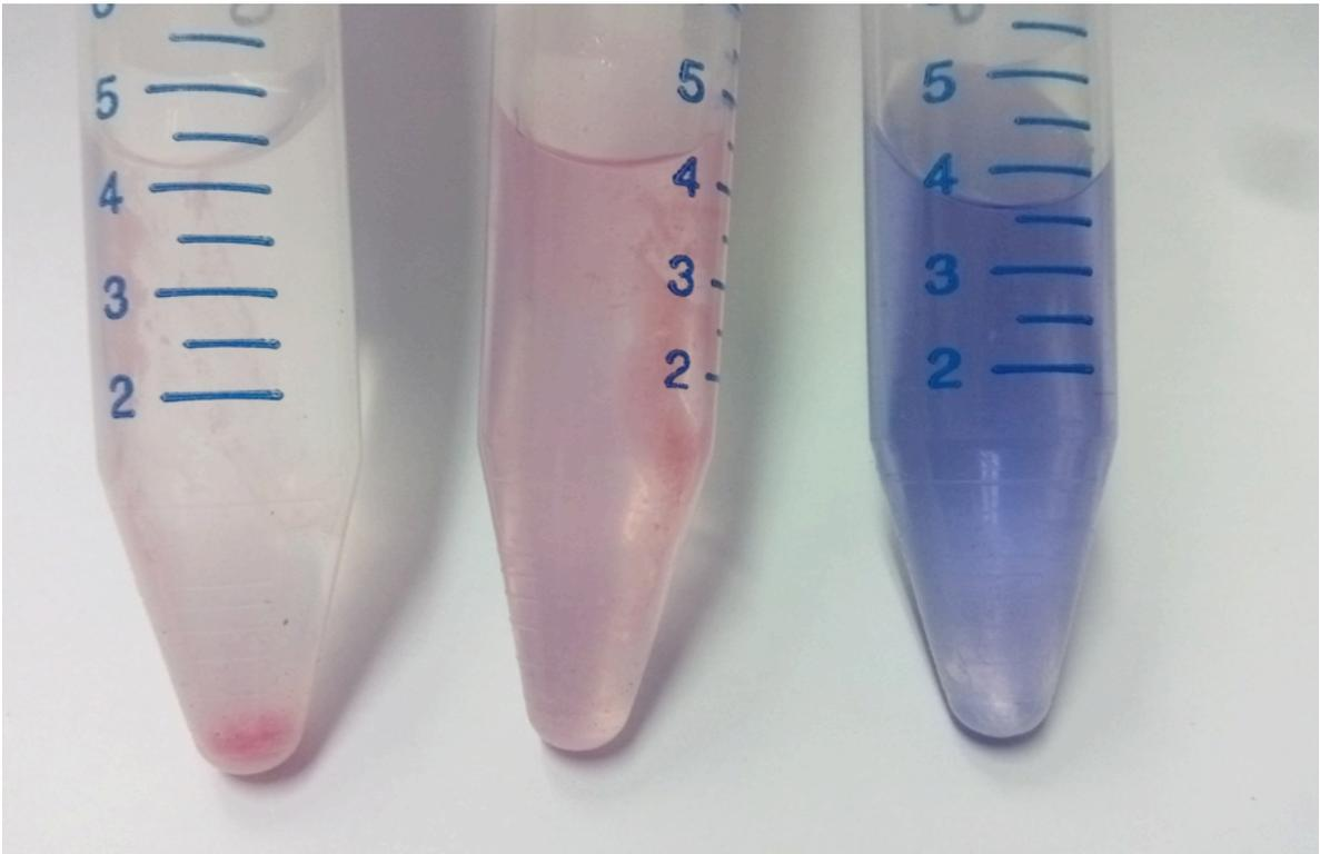
**Figure 7.** Image of DOX conjugated polymers in, a) 0.1 M HCl, b) 12 M HCl, and c) 18.3 M H<sub>2</sub>SO<sub>4</sub>. DOX conjugated polymers that are not dissolved in 0.1 N HCl and 12 M HCl are shown with arrows. Polymer dissolved completely in concentrated H<sub>2</sub>SO<sub>4</sub>.
