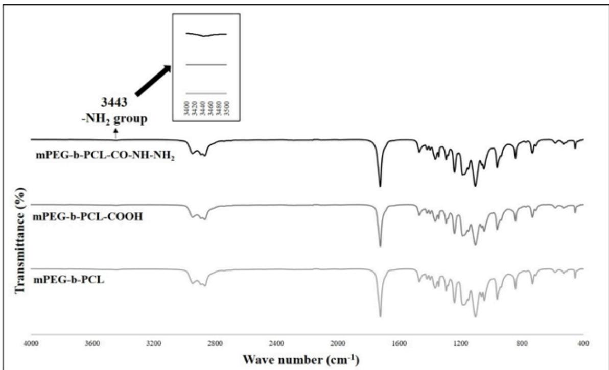
Figure 3. FT-IR spectra of mPEG-b-PCL, mPEG-b-PCL-COOH, mPEG-b-PCL-CO-NH-NH<sub>2</sub>.
