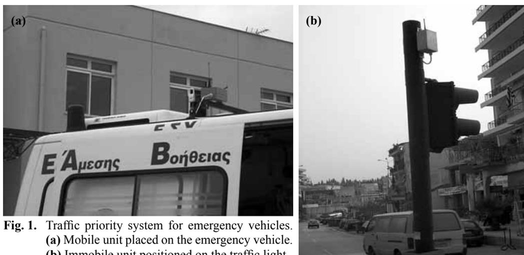
**Fig. 1.** Traffic priority system for emergency vehicles. (a) Mobile unit placed on the emergency vehicle. (b) Immobile unit positioned on the traffic light.
