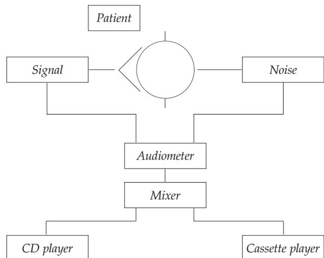
Fig. 1 - The experimental set-up for the speech discrimination measurements.
