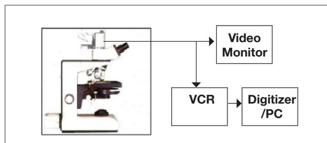
Figure 1. Schematic of smear imaging system
