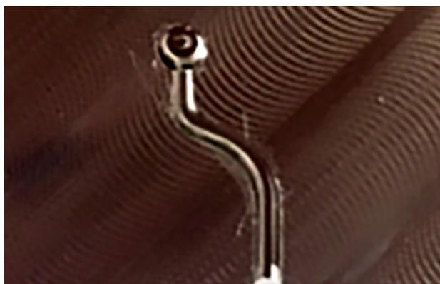
**Fig. 1.** A stainless steel artificial canal with double curvature canal.
